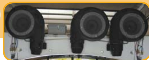
AquaDri E-30i 30 HP on-board dryer, shown here on an AquaJet GT-700, provides fast and thorough drying in bays too short for a freestanding dryer.
